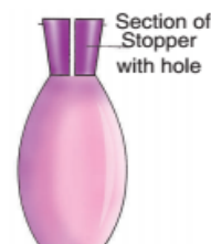
Fig. 1.13. A relative density bottle.
